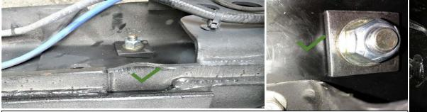
The assembly of bolt and nut through the chassis frame must adhere to certain guidelines. In the event that the hole is situated on a curved surface or where a transition occurs in the frame, it is not recommended to utilize it as a mounting location.
