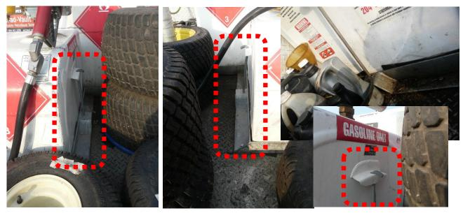
Pictures showing mounting of the transfer/slip tanks in the bed of the flat deck.
