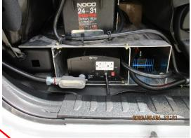
Invertor and deep cycle AGM battery to be install/mounted in front top vertical storage compartment
